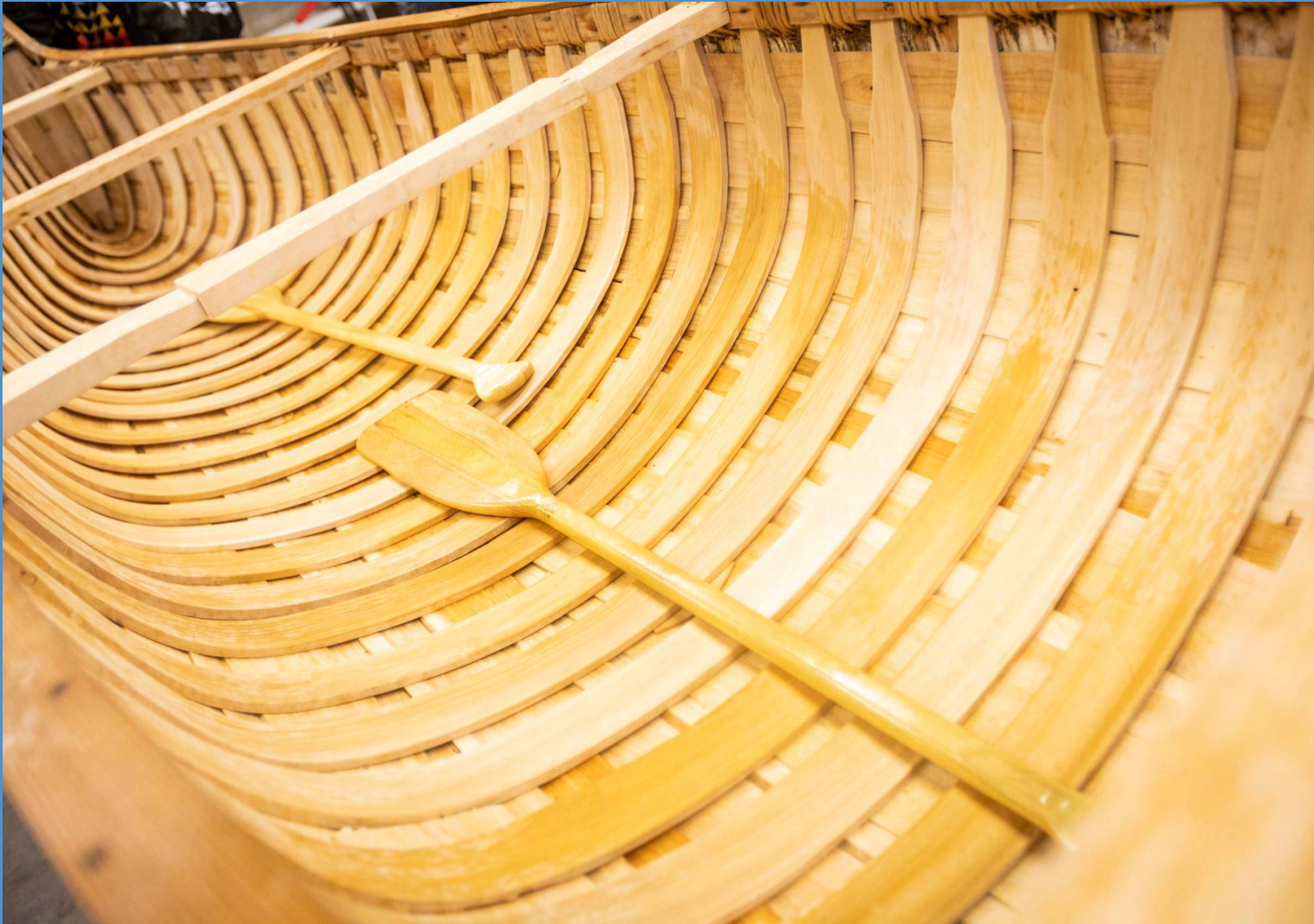
Cedar waaganigaana (ribs) of the birchbark wiigwaasi-jiimaan (canoe).
